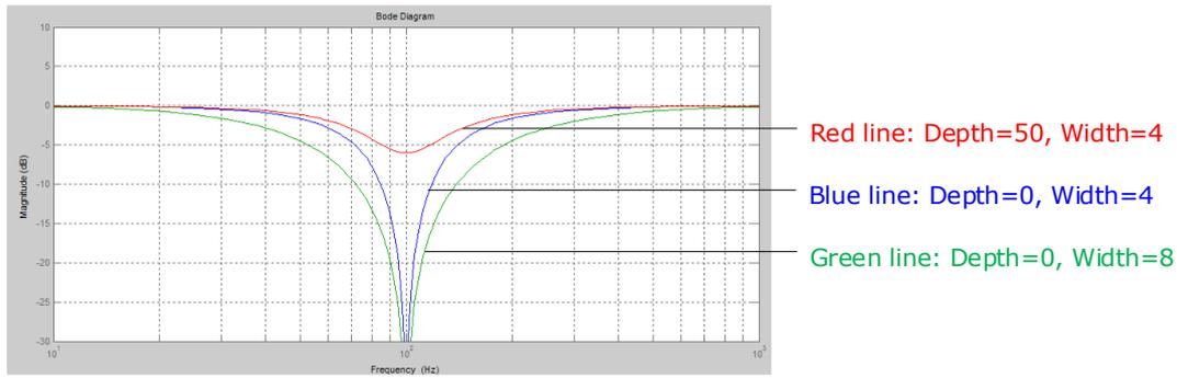
The notch filter parameters can be set from the Tuning page in the drive commissioning screens.
