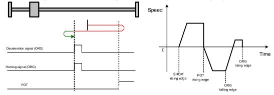
Homing modes 3 and 4, using deceleration point as ORG switch, and origin as Motor's Z signal
