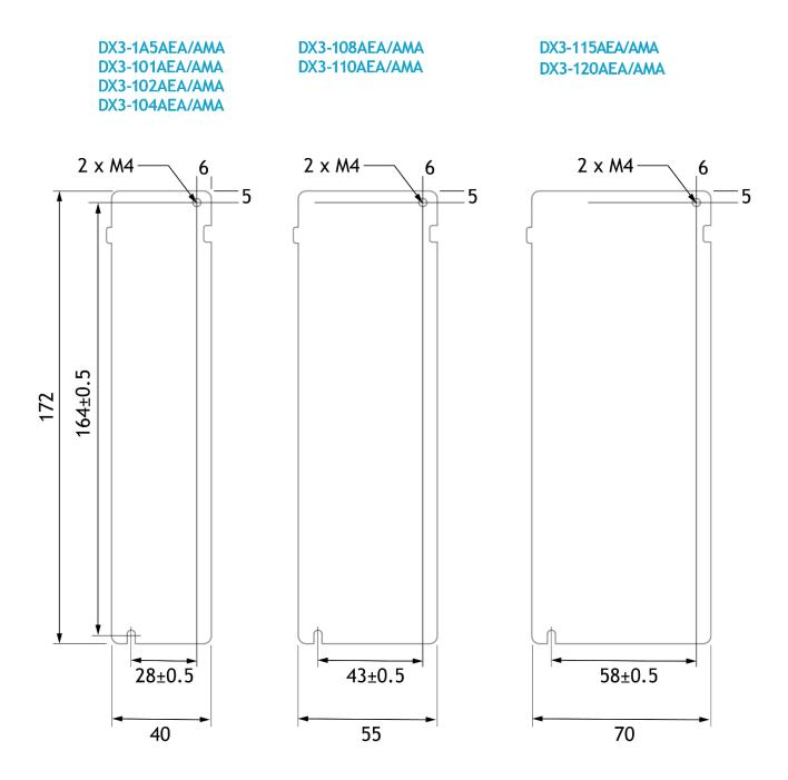
Wiring diagram for mounting holes of 400VAC units
