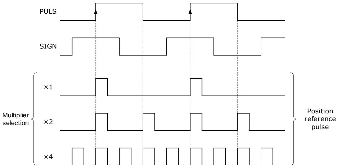
Also, the user can choose whether to invert the PULS signal and SIGN signal using Pn004.3.
