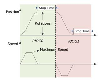
Figure 7-1 Position-speed timing diagram
