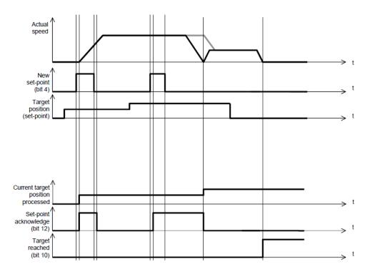
When the speed profile is S (motion\_profile\_type=2), only **Continuous-step setting** is available.  $6083_h$  (profile\_acceleration) limits max acceleration, and 6081h (profile\_velocity) limits max speed. 60A4-01h (VAR Profile\_jerk1) limits the jerk. Only symmetrical S linear is available currently.
