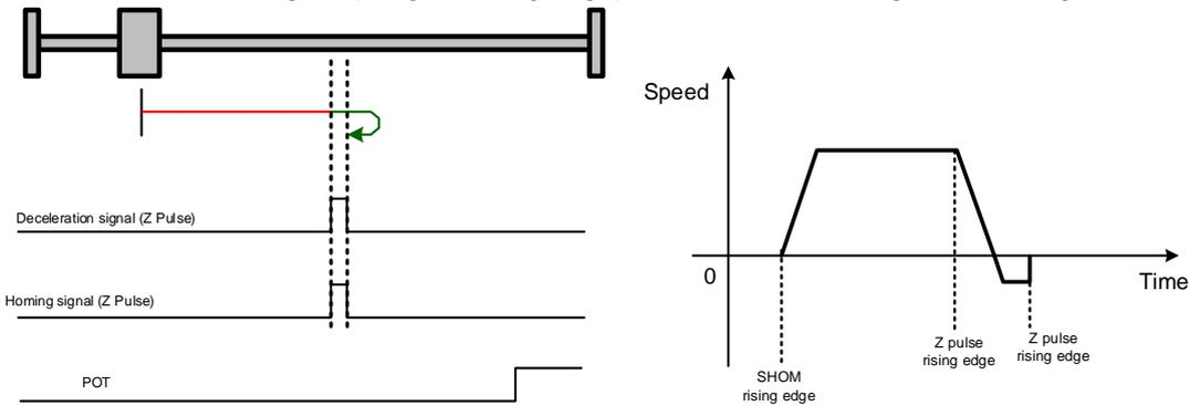
Hit the limit signal before encountering deceleration signal (Z signal rising edge).
