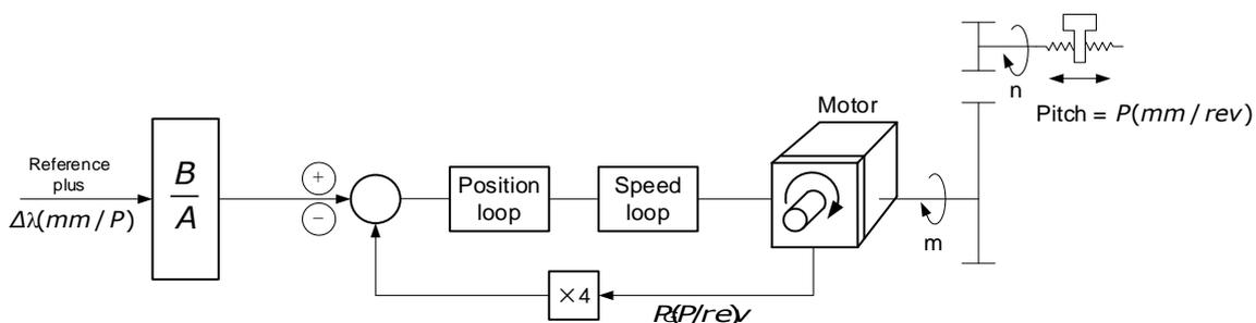
Where:  $\Delta l$  is the reference unit;  $P_G$  is the encoder pulse;  $P$  is the pitch of the ball screw;  $m/n$  is the reduction ratio.
