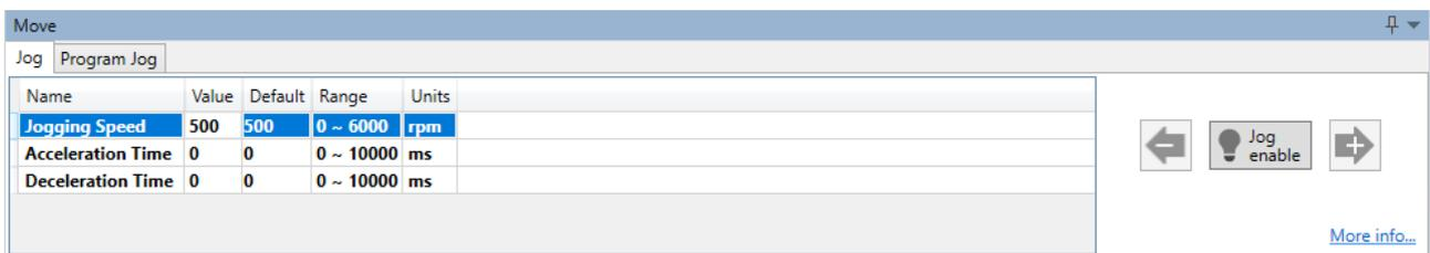
The motion profile is controlled three parameters:
