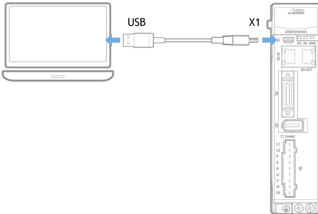
To set up the USB connection, select the external device or network option on the Motion Perfect connection screen. Then select the USB in the connection parameters dropdown menu.
