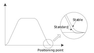
The damping selection can be made from the Tuning page in the drive commissioning screens.
