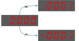
[Note] The adjustment range of the offset is -1024 to 1024.
