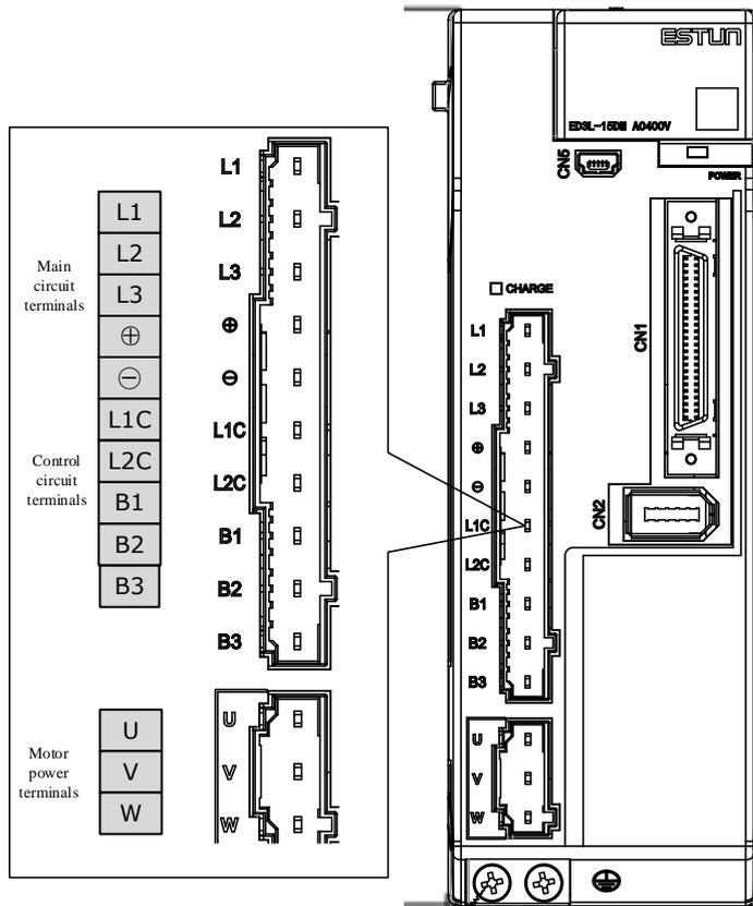
Take for example a product with a power rating of 1kW~1.5kW. Products with power rating from 1.5kW to 3kW are similar in appearance and have the same components
