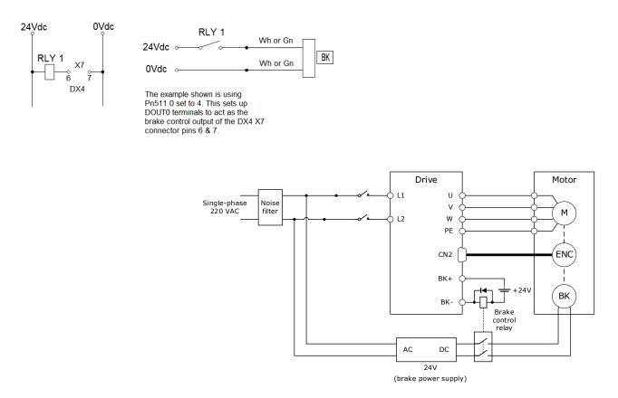
Figure 3-4 Holding brake wiring diagram
