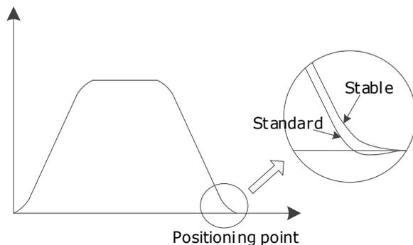
The damping selection can be made from the Tuning page in the drive commissioning screens.
