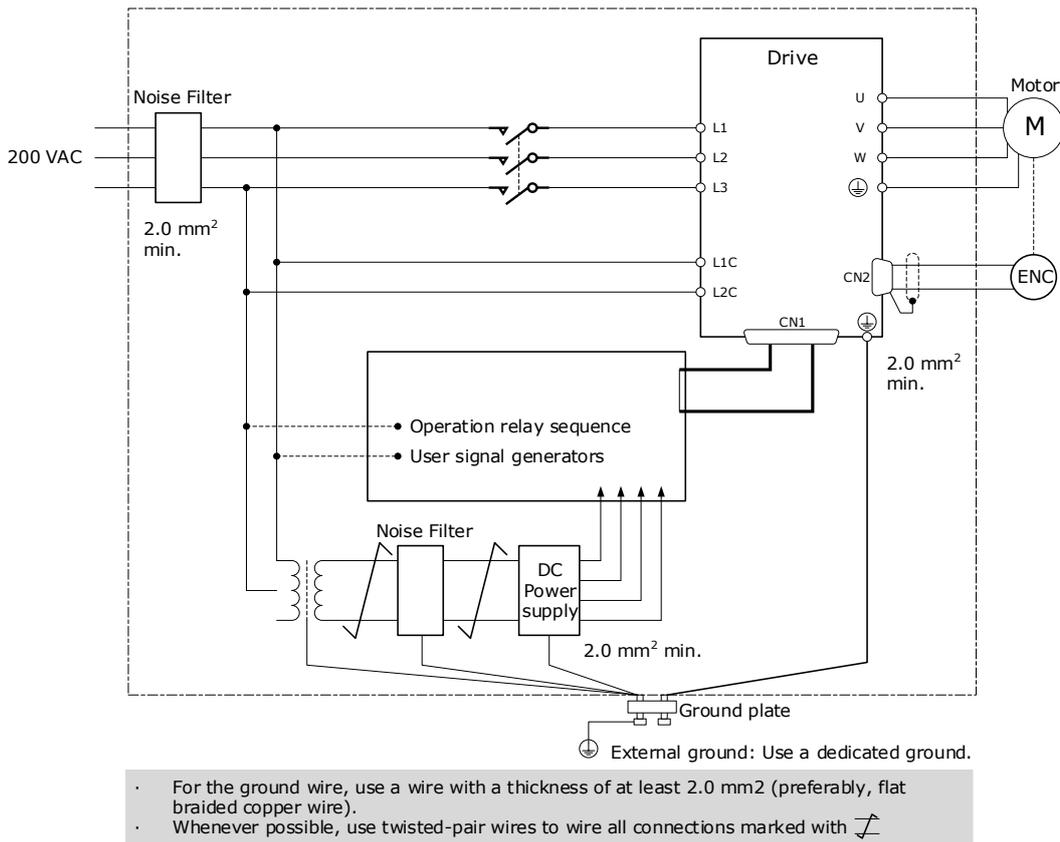
Figure 3-1 Wiring example for countermeasures against noise
