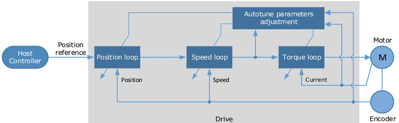
When using the tuning-less function, the following parameters are automatically adjusted.
