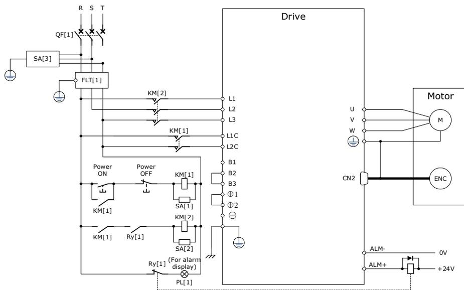
The following figure shows the wiring example for using the single-phase AC input power.
