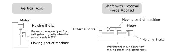
The brake built into a Motor with a Brake is a de-energization brake. It is used only to hold the Motor and cannot be used for braking. Use the holding brake only to hold a Motor that is already stopped.
