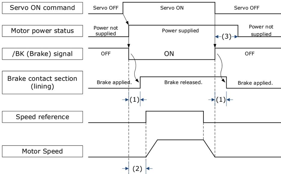
(1): The brake delay times for motors with Holding Brakes.
