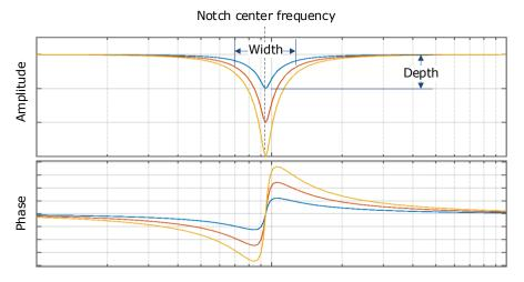
Parameters controlling the operation of notch filter are:
