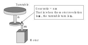
Because the turntable moves in only one direction, the upper limit to the number of revolutions that can be counted by an absolute encoder will eventually be exceeded.
