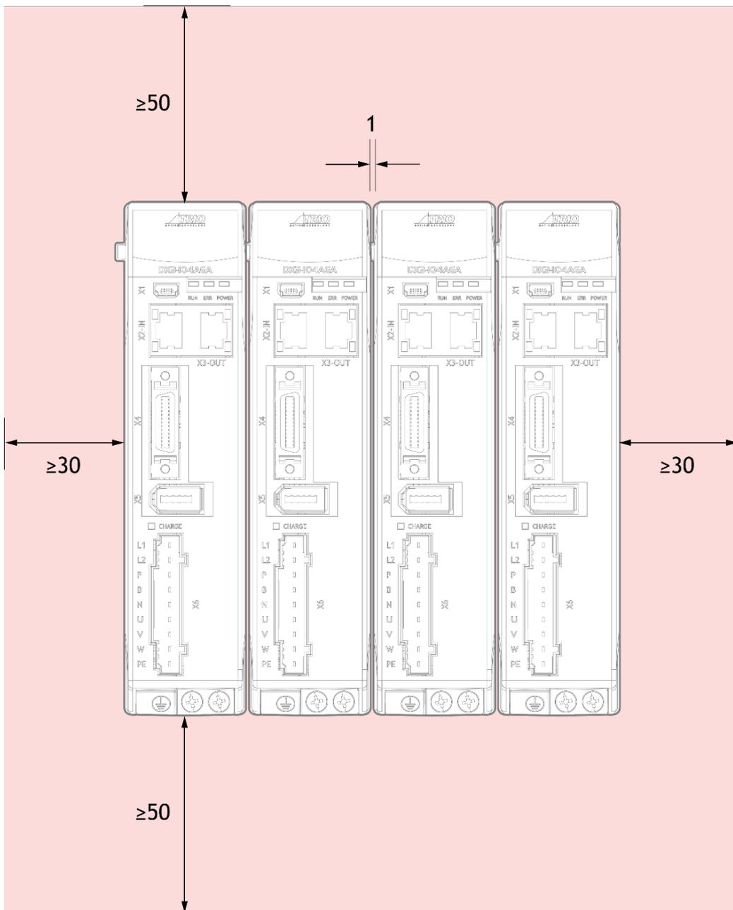
Figure 2-3 Installing multiple Drives in a control cabinet
