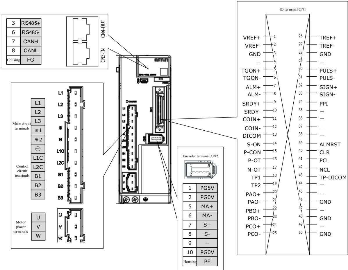
**Rated power from 2kW to 3kW (400VAC)**
