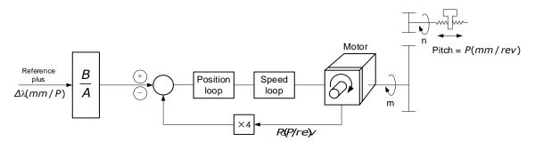
Where:  $\Delta I$  is the reference unit; P\_G is the encoder pulse; P is the pitch of the ball screw; m/n is the reduction ratio.
