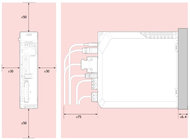
Figure 2-2 Installing a single  $\ensuremath{\mathsf{Drive}}$  in a control cabinet
