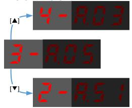
Step 5 Press the [◀] key to return to the display of the Fn000. Press and hold [◀] key for 1 second or more to clear all the alarm trace data.
