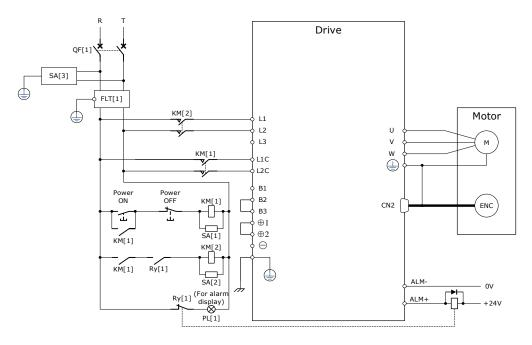
QF[1]: Molded-case circuit breaker SA[3]: Surge Absorber 3 Ry[1]: Relay SA[1]: Surge Absorber 1 FLT[1]: Noise Filter PL[1]: Indicator lamp SA[2]: Surge Absorber 2
