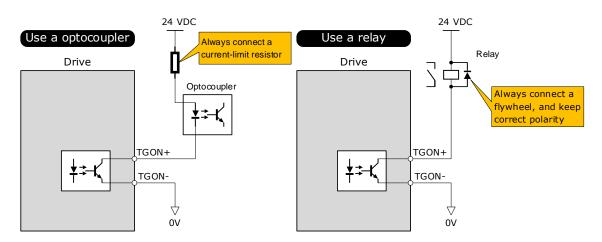
Figure 3-3 TGON wiring diagram
