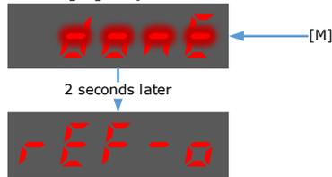
Step 7 Press the [◀] key to return to the display of the Fn003.
