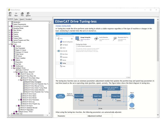
The commissioning screens for the Drive are listed below. The menu is split into 2 groups, Drive and Motor. The Drive screens are for status and operations that are not necessarily axis specific. The Motor screens show detail that is axis specific.
