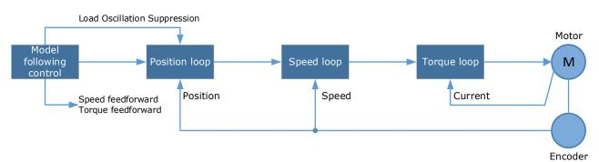
This function is based on the Model Following Control (8.8) and enabled via Pn150.
