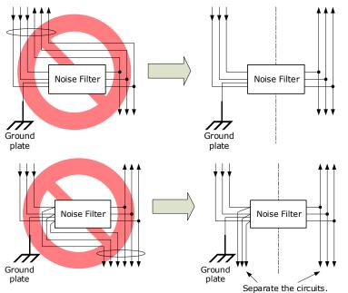
• Separate the Noise Filter ground wire from the output lines. Do not place the Noise Filter ground wire, output lines, and other signal lines in the same duct or bundle them together.
