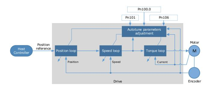
One-Parameter Auto Tuning requires an inertia measurement of the load. The drive can measure the load inertia using the Inertia Detection tool, which can be launched from the Tuning page in the drive commissioning screens
