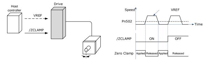
Adjust the position loop gain in Pn104 (position loop gain) if the servomotor oscillates in the zero clamp state. If the gain switching function is used, adjusting Pn109 (2nd position loop gain) is also required.
