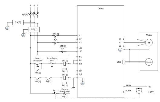
QF[1]: Circuit breakerSA[1]: Surge Absorber 1SA[2]: Surge Absorber 2SA[3]: Surge Absorber 3FLT[1]: Noise FilterKM[1]: Magnetic Contactor (for control power supply)KM[2]: Magnetic Contactor (for main circuit power supply)Ry[1]: RelayPL[1]: Indicator lamp for display
