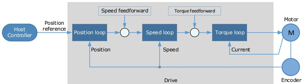
In general, the differential of the position reference is used as the feedforward. This is known as an internal feedforward reference and is the default mode of operation. Other options are available for generating the feedforward reference.
