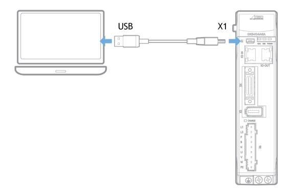
To set up the USB connection, select the external device or network option on the Motion Perfect connection screen. Then select the USB in the connection parameters dropdown menu.
