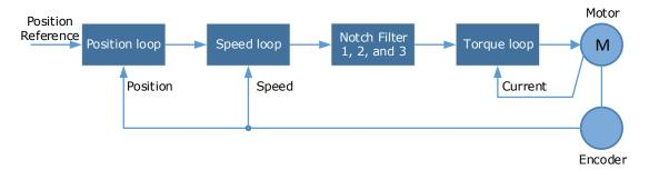
The diagram below shows the relevant parameters for the notch filter.
