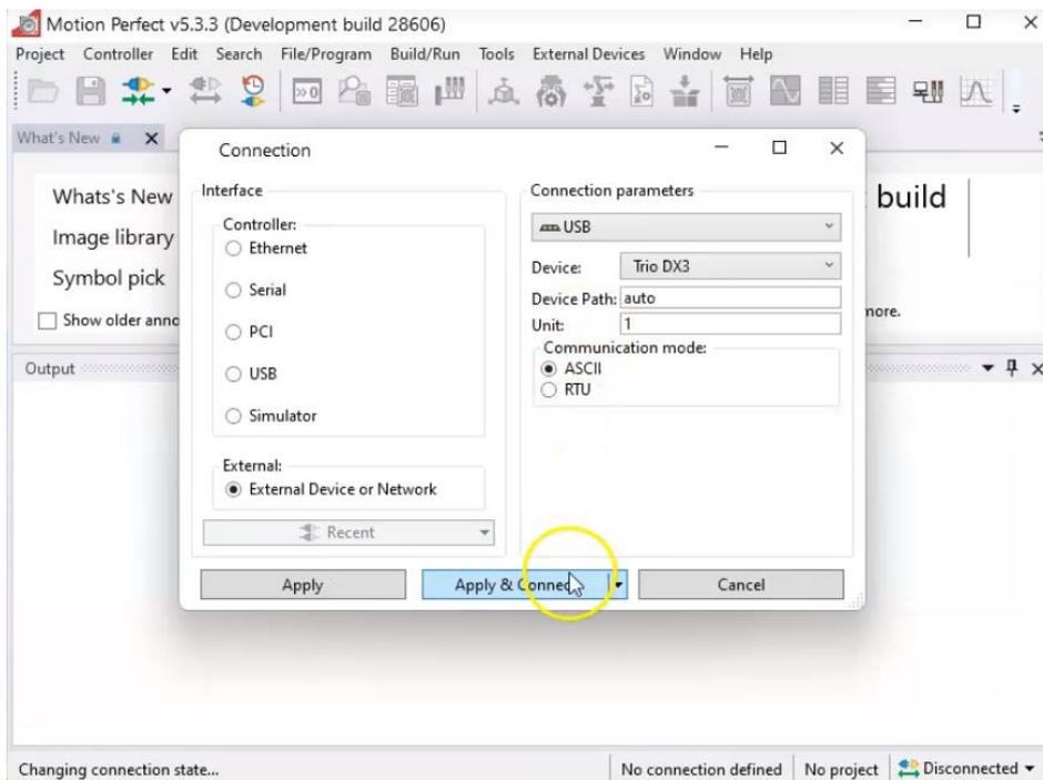
The first time you connect through USB on a computer, Motion Perfect will need to install the necessary drivers through a pop up if it detects they aren't yet installed.
