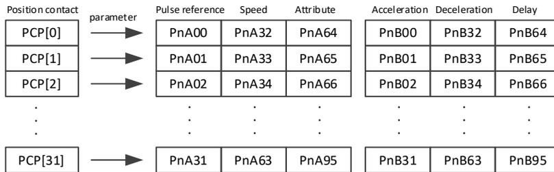
The pulse reference defines the number of pulses of the contact, the speed defines the running speed of the contact, the attributes defines the motion attribute of contact, the acceleration and jerk define the acceleration/deceleration of the contact, and the delay defines the delay time after the contact reference is sent.
