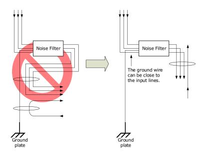
• Connect the Noise Filter ground wire directly to the grounding plate. Do not connect the Noise Filter ground wire to other ground wires.
