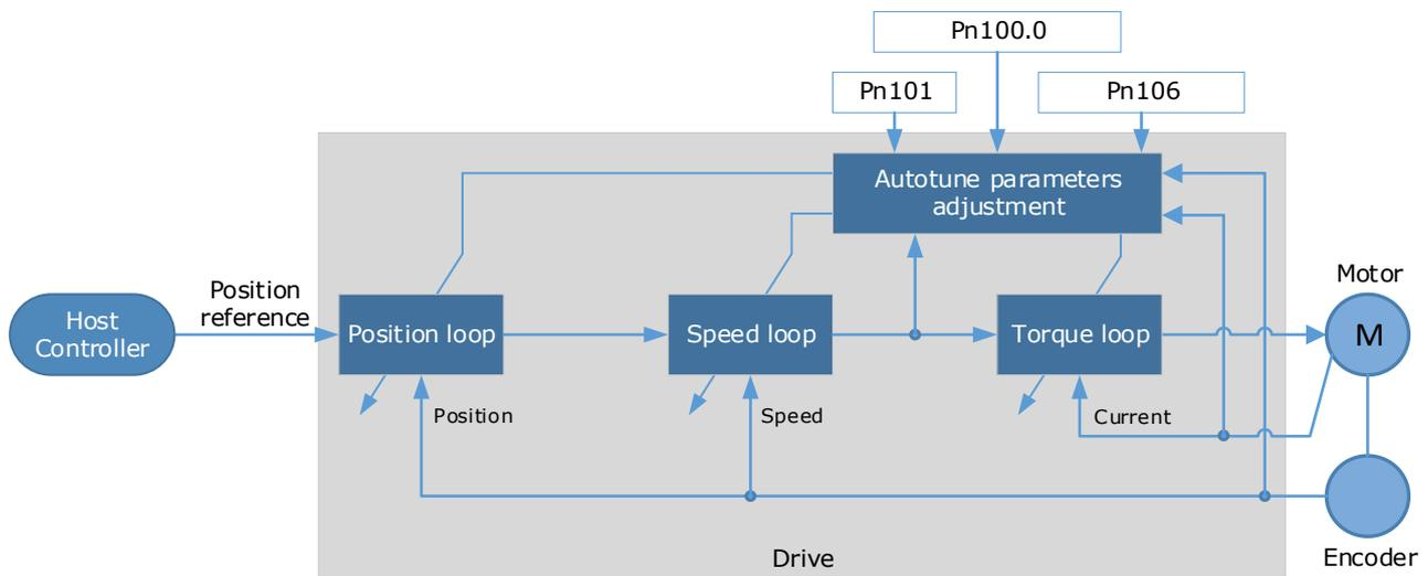
One-Parameter Auto Tuning requires an inertia measurement of the load. The drive can measure the load inertia using the Inertia Detection tool, which can be launched from the Tuning page in the drive commissioning screens
