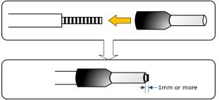
Step 4 Crimp the cable that has been inserted into the ferrule, and cut off the cable conductor portion protruding from the ferrule (The allowable protruding length after cutting should not be more than 0.5 mm).
