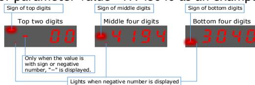
The example below shows how to change parameter Pn504 (Deviation Counter Overflow Alarm) from 41943040 to 42943240.
