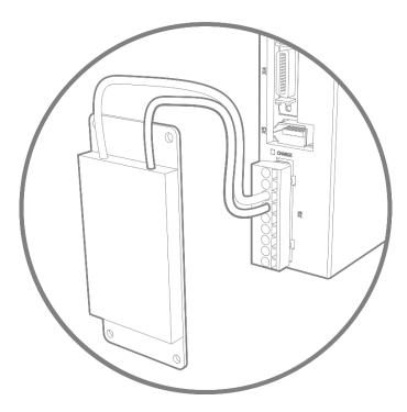
Connect the external regenerative resistor as following to avoid damaging the drive or malfunction.
