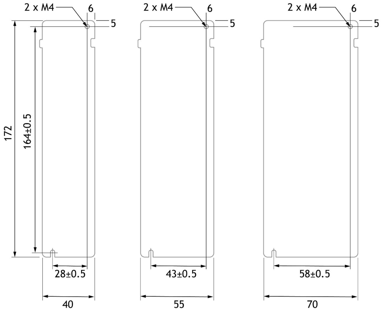
Wiring diagram for mounting holes of 400VAC units
