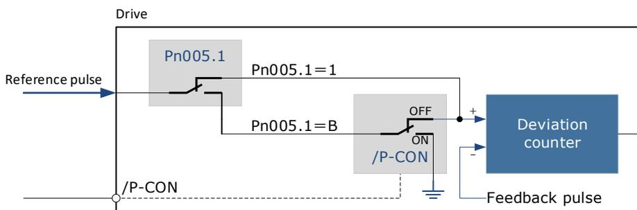
Inhibit (INHIBIT) is switched via /P-CON signal:
