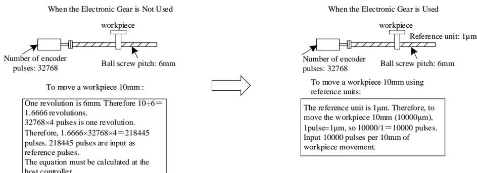
If the mechanical reduction ratio between the motor shaft and the load side is set to  $m/n$ , the setting value of the electronic gear ratio can be calculated according to following formula. (When the servomotor rotates  $m$  revolutions, the load shaft rotates  $n$  revolutions)
