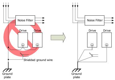
• If a Noise Filter is located inside a control panel, first connect the Noise Filter ground wire and the ground wires from other devices inside the control panel to the grounding plate for the control panel, then ground the plate.
