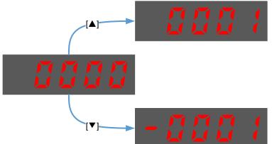
**NOTE:** the offset can be adjusted from -1024 to 1024.
