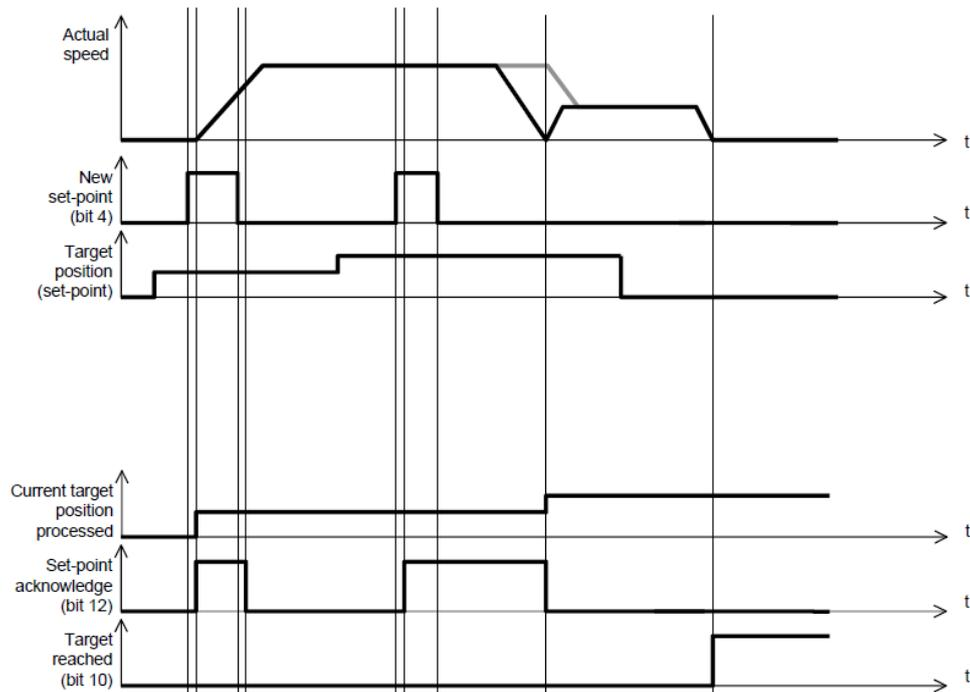
When the speed profile is S (motion\_profile\_type=2), only **Continuous-step setting** is available. 6083<sub>h</sub> (profile\_acceleration) limits max acceleration, and 6081<sub>h</sub> (profile\_velocity) limits max speed. 60A4-01<sub>h</sub> (VAR Profile\_jerk1) limits the jerk. Only symmetrical S linear is available currently.
