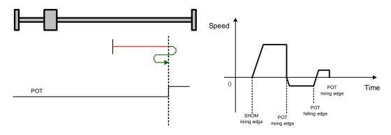
Homing modes 9 and 0, using deceleration point as overtravel switch, and origin as motor's Z signal
