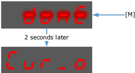
Step 5 Press the [◀] key to return to the display of the Fn005.
