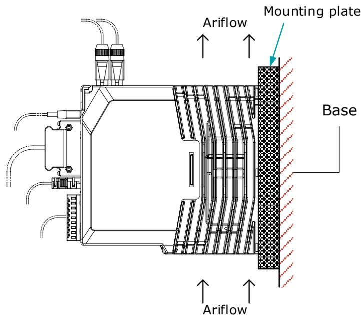
Figure 2-1 Base-mounted diagram
