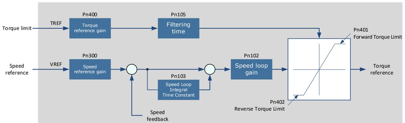
[Note] There is no issue with input voltage polarity of the Analogue voltage reference for torque limiting. The absolute values of both + and - voltages are input, and a torque limit value corresponding to that absolute value is applied in the forward or reverse direction.
