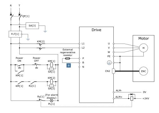
QF[1]: Molded-case circuit breakerSA[1]: Surge Absorber 1SA[3]: Surge Absorber 3FLT[1]: Noise FilterRy[1]: RelayPL[1]: Indicator lampKM[1]: Magnetic Contactor (for control power supply)KM[2]: Magnetic Contactor (for main circuit power supply)
