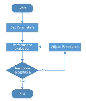
There are various indicators used to evaluate servo performance including bandwidth, response time, overshoot, steady state error, anti-load disturbance, speed ripple fluctuation, torque ripple, etc. The importance of these will depending on the application.
