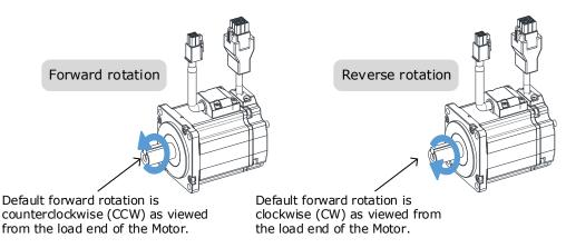
The rotation direction of the Motor can be changed by setting the Motor Direction from the Basic Setup page in the drive commissioning screens. The figure above shows the default setting.
