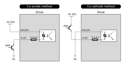
Figure 3-2 P-OT wiring diagram
