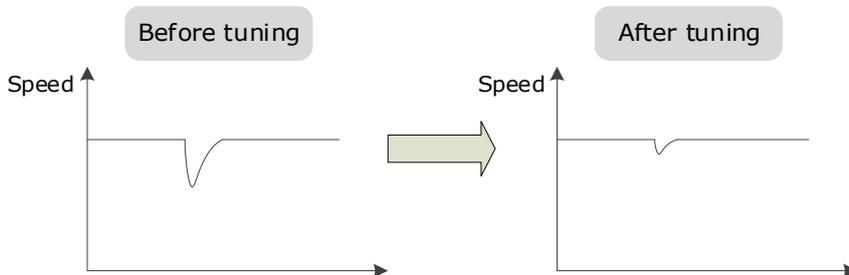
Tuning the load torque compensation function can be used to improve the anti-load disturbance performance, considering that the reference response performance and the load disturbance resistance cannot be balanced.
