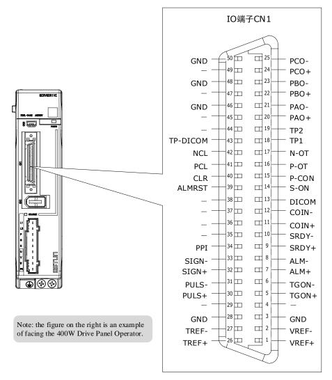
• The signal definitions for the IO signals of all drives are the same.
