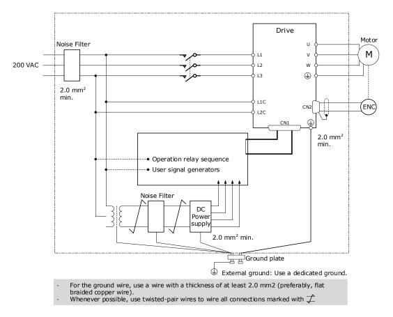
Figure 3-1 Wiring example for countermeasures against noise
