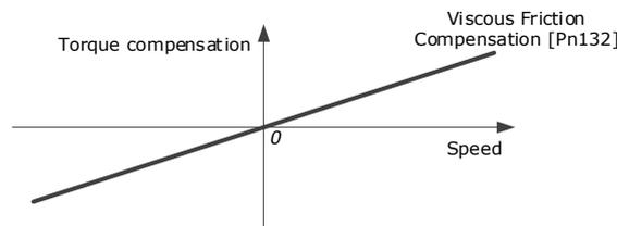
As the speed increases, so the viscous friction compensation increases with a rate defined by the Viscous Friction Compensation parameter.
