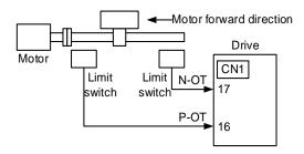
Figure 5-1 Wiring diagram for the overtravel
